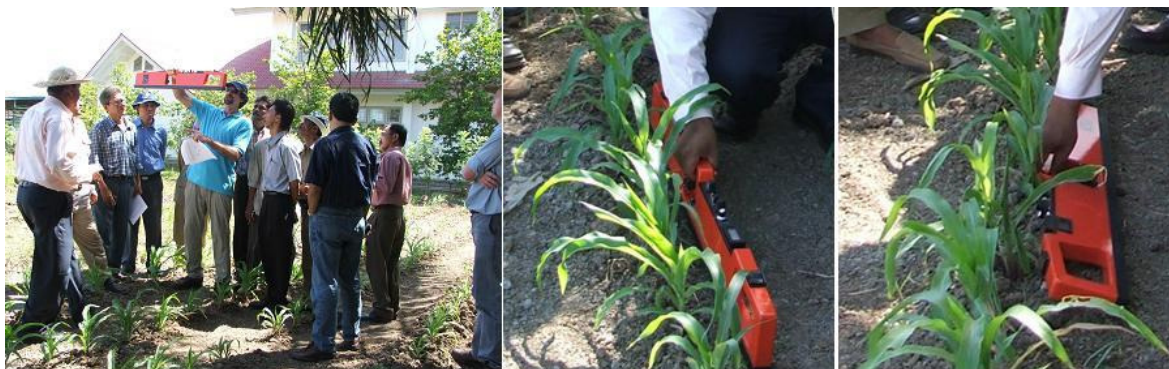
Figure 3. Training of agricultural research staff in Aceh to use the EM38 instrument (left), using EM38 in a vertical dipole orientation (middle), and using the EM38 instrument in a horizontal dipole orientation (right)
